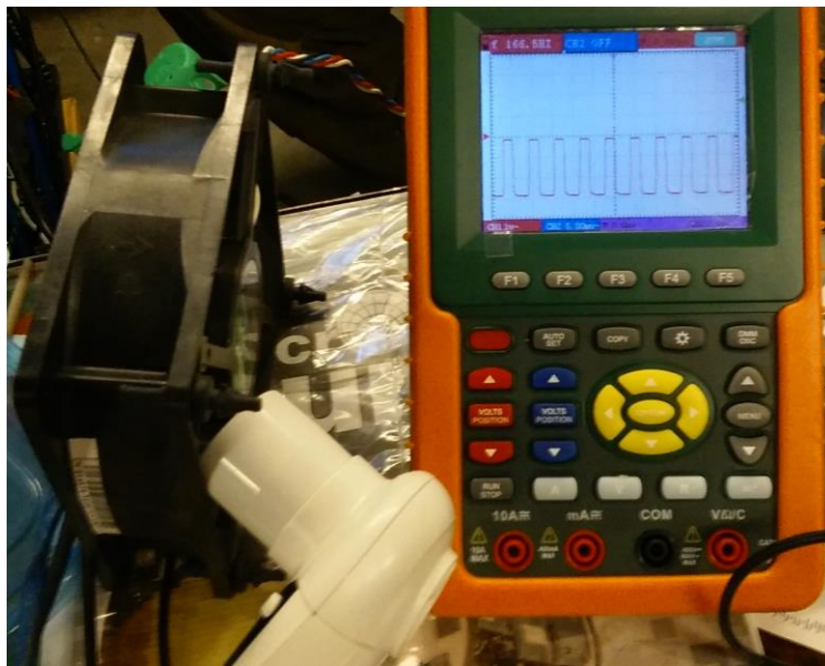
Figure 8: The Peak Expiratory Flow meter was placed in front of a constant speed air source and the signal was analyzed during the prototype development.
